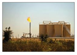
receives are for flaring casinghead gas. In new areas of exploration, pipeline connections are not typically constructed until after a well is completed and a determination is made about the well's productive capability.
